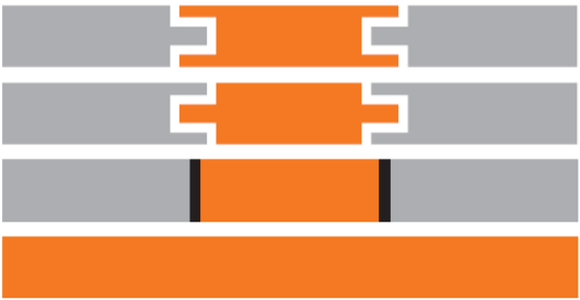
Figure 11: Closed, complete obstruction to the (Interim) removal of products or elements.
