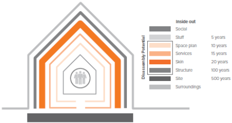
Figure 4: Disassembly potential within the Layers of Brand. Adapted from 'How building learn' by Brand, S., 1994.
